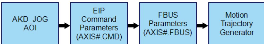
In Position operation mode the AXIS#.EIP parameter values are passed to the corresponding AXIS#.FBUS parameters.
