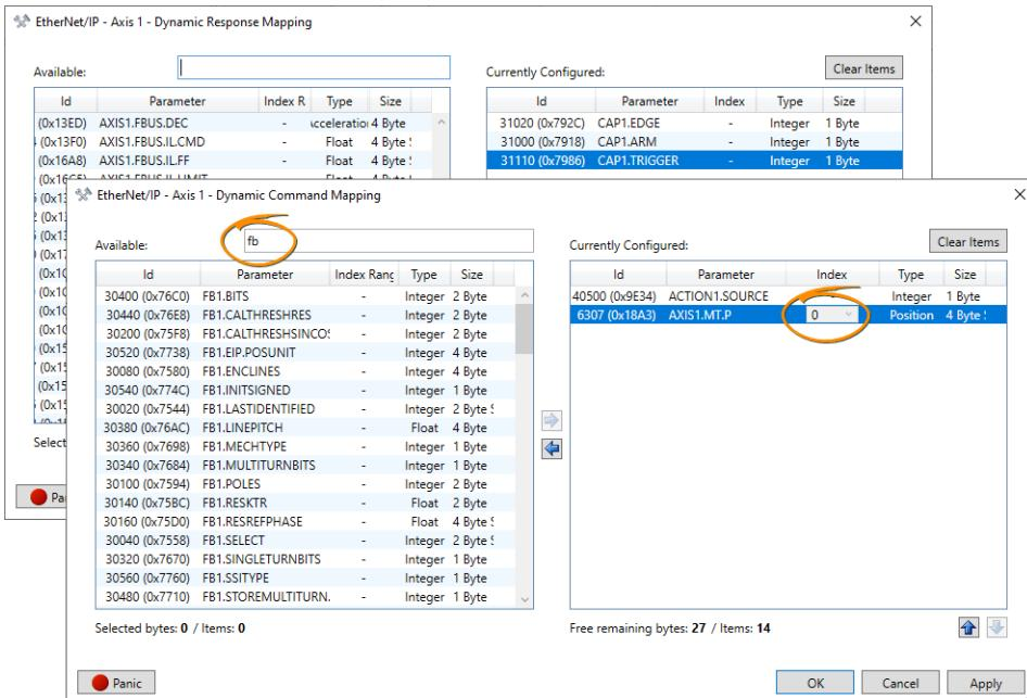
3. Select the desired parameter and then press the right arrow key in the center of the screen to move the parameter into the "Currently Configured" list.
