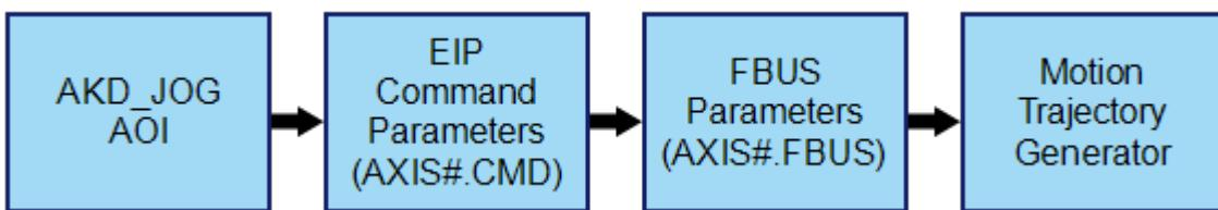
The AXIS#.EIP parameter values are passed to the drive as follows:
