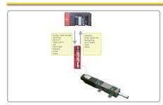
Position Table can be used for motion control by digital input and output signals of host controller. You can operate the motor directly by sending the position table number, start/stop, origin search and other digital input values from a PLC. The PLC can monitor the In-Position, origin search, moving/stop, servo ready and other digital output signals from a drive. A Maximum of 256 positioning points can be set from PLC.
