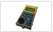
Using the teaching pendant only, where the location of a table of data creation and editing of the program, run, jog function, parameter editing and monitoring functions can be performed.
