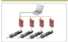
A maximum of 16 axis can be operated from a PC through RS-485 communication, All of the motion canditions are set through the network and saved in Flash ROM as a parameter. Motion Librart(DLL) is provided for programming under windows 2000/XP.
