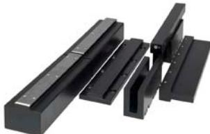
Series SLM contains iron core, 3-phase, encoder commutated synchronous linear motors from 220 to 1450 N peak force. Series SLME provides ironless direct linear motors from 150 N to 400 N peak force.
