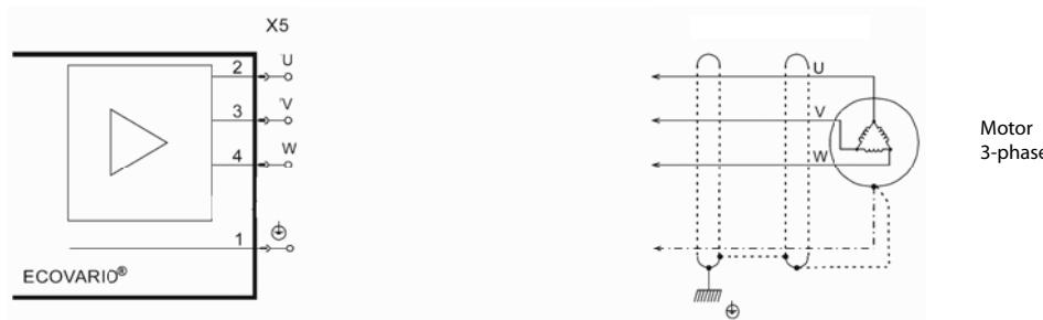
Fig. 6.9 X5: Example for connection with standard cable, e.g.
