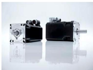
The motor ranges 60B and 80B contain rotative 2-phase, encoder-commutated low-pole synchronous motors with flanges of 60 mm and 80 mm and holding torques between 0.6 and 3 Nm. The motor ranges 60C and 80C are 3-phase with holding torques between 0,93 and 3,5 Nm.
