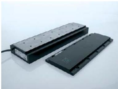
Series SLM contains iron core, 2-phase, encoder commutated synchronous linear motors from 220 N to 1650 N peak force.
