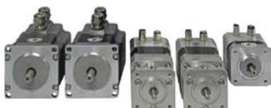
The motor ranges 17H and 23S contain rotative 2-phase, encoder-commutated, high-pole synchronous motors with flanges of 42 mm and 56 mm and holding torques between 0.2 and 3.8 Nm.
