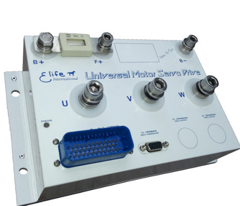
(a) Electrical Box Version Size: 250x150x75 mm
