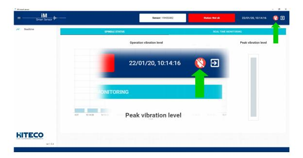
By applying increasing vibration level to iM Smart Sensor, the HMI shows that increase, in **spindle status** window, with higher and orange/red color bars. Also the **Status button** turns from green to red because the vibration level overcome the dangerous level.
