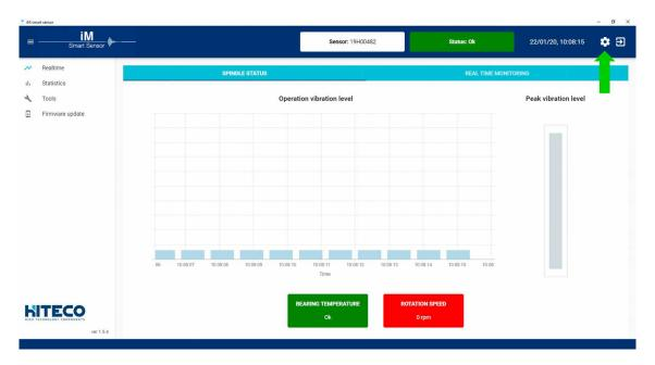
By clicking on it a new window pops up where it's possible to add to the HMI a new iM Smart Sensor. On the "+" box the HMI adds a new sensor to its interface.
