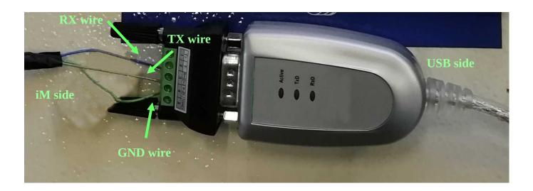
The sensor power supply is connected to the s3 sensor power supply and share the gnd wire with it in order to acquire the inspeed signal. Even if the s3 sensor is not present in the spindle or is not utilized his wires/pin have to be power supplied to get iM Smart Sensor active.
