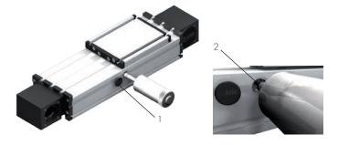
Lubrication is effected by an oiled felt insert. The felt can be re-oiled through lubrication nipples attached laterally to the ends of the roller packs.
