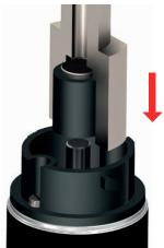
Press the hub with magnet onto the motor shaft by the centering gauge
