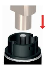
Align the base plate to the motor shaft by using the centering gauge
