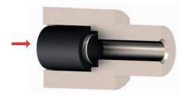
Set the hub with magnet into the centering gauge
