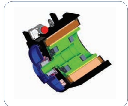
Design of a Cartridge DDR motor (CDDR)
